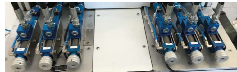
Example of volumetric dosers battery, to make multiple doses on assembling lines both automatic and semi-automatic.
