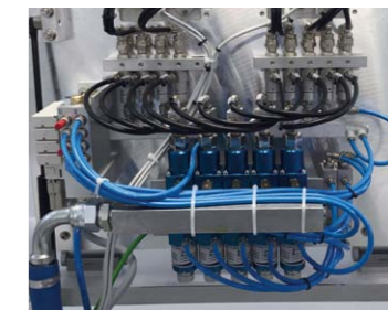
Example of volumetric dosers battery, to make multiple doses on assembling lines both automatic and semi-automatic.
